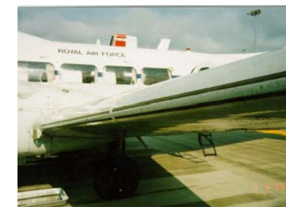
TKS Strip Panels on a DeHavilland Dove
