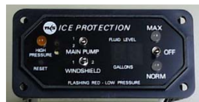
Known Icing Style Control Panel
