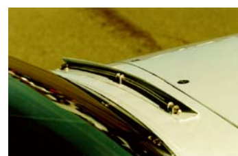
Windshield Spraybar and Deflector on Mooney
