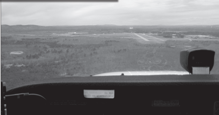
Left: Flying runway heading to the airport is really flying to the airport reference point, which may not be on a runway. Also, the GPS computes magnetic variation on the fly and may not completely agree with the magnetic alignment of the runway. So, even if you input the precise magnetic alignment of the runway, you may be paralleling the runway or on a slight angle.
